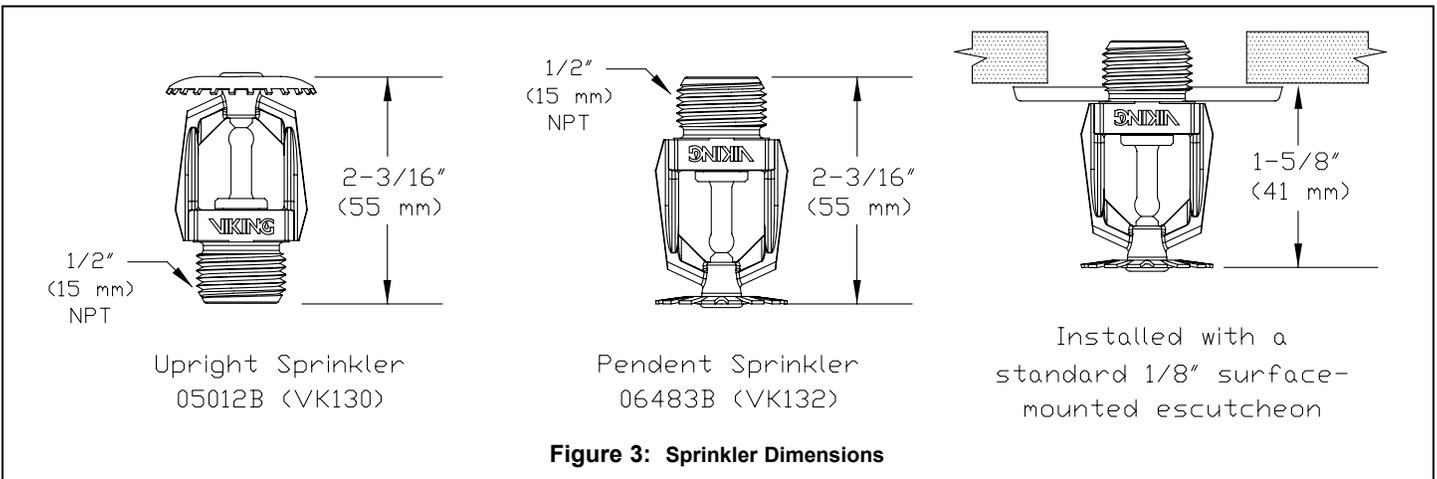
Figure 3: Sprinkler Dimensions
